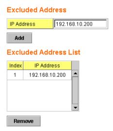
**Manual Binding:** *JetNet 4510* provides a MAC address and IP address binding and removing function. You can type in the specified IP and MAC address then click **Add** to add a new MAC&IP address binding rule for a specified link partner, like PLC or any device without **DHCP client** function. To remove from the binding list, just select the rule to remove and click **Remove**.
