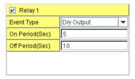
**How to turn On/Off the other device**: Type "1" into the "On period" field and "0" into "Off Period" field and apply the setting, then it t will be trigger to form as a close circuit. To turn off the relay, just type "0" into the "On period" field and "1" into "Off Period" field and apply the setting, the relay will be trigger to form as a open circuit.
