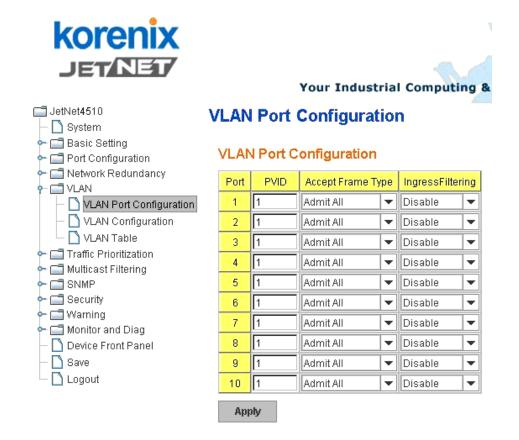
**PVID:** The abbreviation of the **Port VLAN ID**. Enter port VLAN ID here. PVID allows the switches to identify which port belongs to which VLAN. To keep things simple, it is recommended that PVID is equivalent to VLAN IDs.
