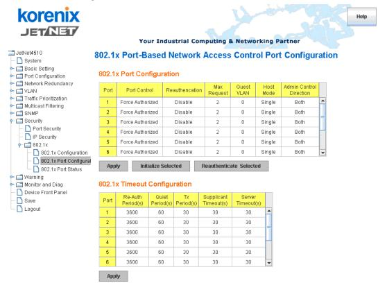
**Port control:** Force Authenorized means this port is Authenorized, the data is free to in/out. Force unauthenorized just opposite, the port is blocked. If users want to control this port with Radius Server, please select Auto for port control.
