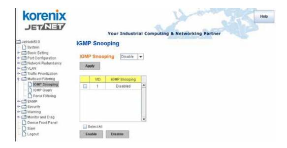
**IGMP Snooping Table**: In the table, you can see multicast group IP address, VLAN ID it belongs to, and member ports of the multicast group. *JetNet 4510* supports 256 multicast groups. Click on **Reload** to refresh the table.
