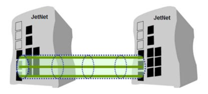
There are some different descriptions for the port trunking. Different manufacturers may use different descriptions for their products, like Link Aggregation Group (LAG), Link Aggregation Control Protocol, Ethernet Trunk, EtherChannel...etc. Most of the implementations now conform to IEEE standard, 802.3ad.
