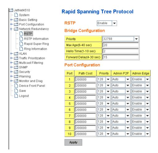
**RSTP Mode:** You must first enable STP/RSTP mode, before configuring any related parameters. Parameter settings required for both STP and RSTP are the same. Note that 802.1d refers to STP mode, while 802.1w refers to faster RSTP mode.
