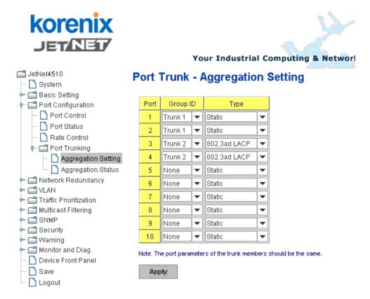
**Trunk Size:** The switch can support up to 5 trunk groups. Each trunk group can support up to 8 member ports. Since the member ports should use same speed/duplex, max groups for 100M ports would be 10.
