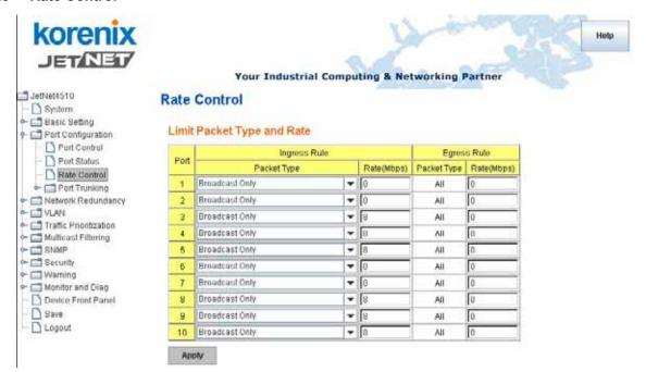
Rate limiting is a form of flow control used to enforce a strict bandwidth limit at a port. You can program separate transmit (Egress Rule) and receive (Ingress Rule) rate limits at each port, and even apply the limit to certain packet types as described below.
