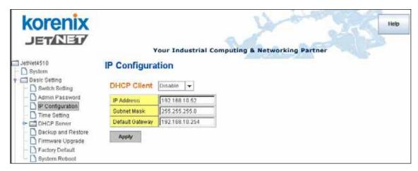
**DHCP Client**: You can select to **Enable** or **Disable** DHCP Client function. When DHCP Client function is enabled, an IP address will be assigned to the switch from the network's DHCP server. In this mode, the default IP address will therefore be replaced by the one assigned by DHCP server. If DHCP Client is disabled, then the IP address that you specified will be used instead.
