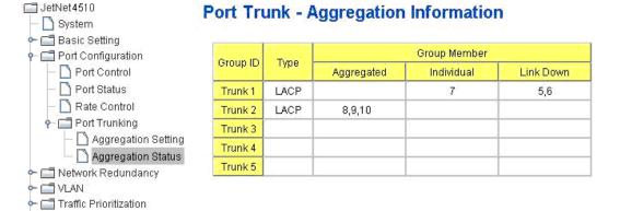
Group ID: Display Trunk 1 to Trunk 5 set up in Aggregation Setting.
