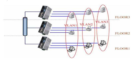
VLAN Configuration group enables you to Add/Remove VLAN, configure port Ingress/Egress parameters and view VLAN table.
