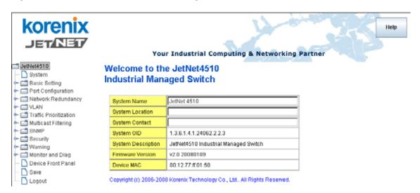
**System Name**: You can assign a name to the device. The available characters you can input is 64. After you configure the name, CLI system will select the first 12 characters as the name in CLI system.
