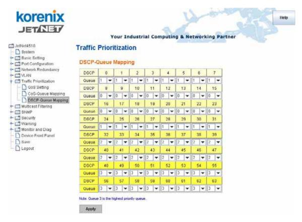
After configuration, press Apply to enable the settings.
