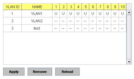
Figure 4.5.2.4 Configure Egress rule of the ports.
