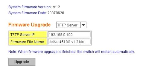
Type the IP address of TFTP Server and Firmware File Name. Then click on **Upgrade** to start the process.
