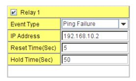
How to configure: After selecting Ping Failure event type, the system will turn Relay Output to short state and continuously ping the target device. When the ping failure occurred, the switch will turn the Relay Output to open state for a period of Reset Time.
