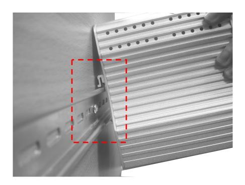
2. Lightly push the bottom of DIN-Rail clip into the track.
