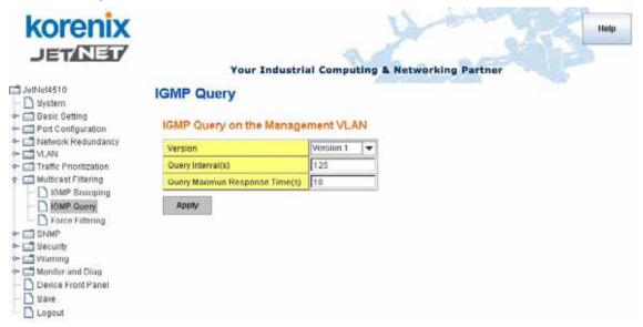
This page allows users to configure **IGMP Query** feature. Since *JetNet 4510* can only be configured by member ports of the management VLAN, IGMP Query can only be enabled on the management VLAN. If you want to run IGMP Snooping feature in several VLANs, you should notice that whether each VLAN has its own IGMP Querier first.
