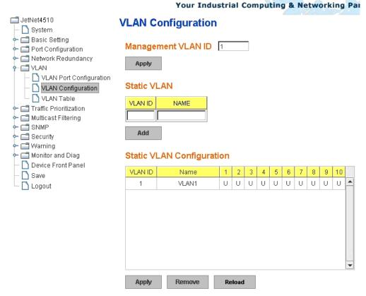
**Management VLAN ID:** The switch supports management VLAN. The management VLAN ID is the VLAN ID of the CPU interface so that only member ports of the management VLAN can ping and access the switch. The default management VLAN ID is 1.
