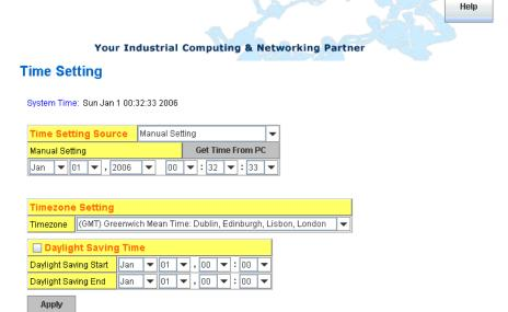
**Manual Setting**: User can select Manual setting to change time as user want. User also can click the button "Get Time from PC" to get PC's time setting for switch.
