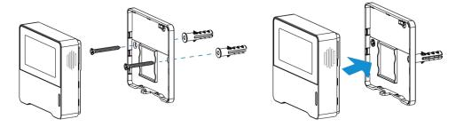
2. Fix the bottom of the device to the rear cover with the theft-deterring screw.
