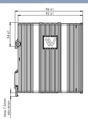
$\textbf{Dimension W x H x D} \quad 52 \times 100 \times 101 \text{ mm} (2.04 \times 3.93 \times 3.97 \text{ in})$
