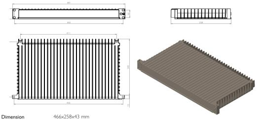
Weight 3,8 kg Degree of protection IP 40
